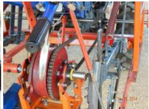
The LH picture shows a rear view of a 'rope trip lift'. The rope trip lift is also shown in RH picture. This drives from the countershaft above the front tool bar.
