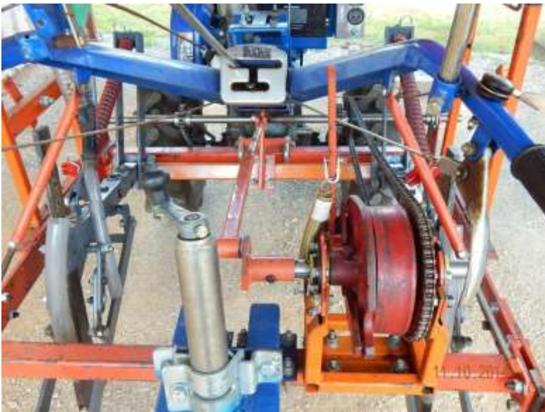
The LH picture shows a rear view of a 'rope trip lift'. The rope trip lift is also shown in RH picture. This drives from the countershaft above the front tool bar.
