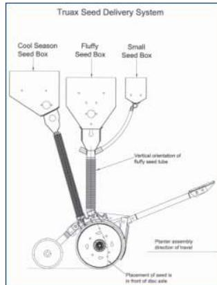
Seed from all boxes is delivered between the double disc openers. The rolling disc opener carries the seed into the soil for proper placement and optimal seed-to-soil contact. A guard in front of the disc openers reduces plugging problems. Truax EZ-Off Depth Bands on every disc control planting depth. Four sizes are available to accommodate planting depths of different crops. Each opener is independently supported with down pressure springs.
