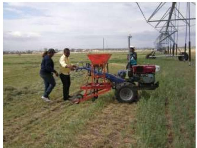
The unit was set up in a two row configuration, for row crop planting, although it is capable of planting up to four rows of close drilled crops. It had no difficulty planting into the light residue conditions with cut lucerne plants
