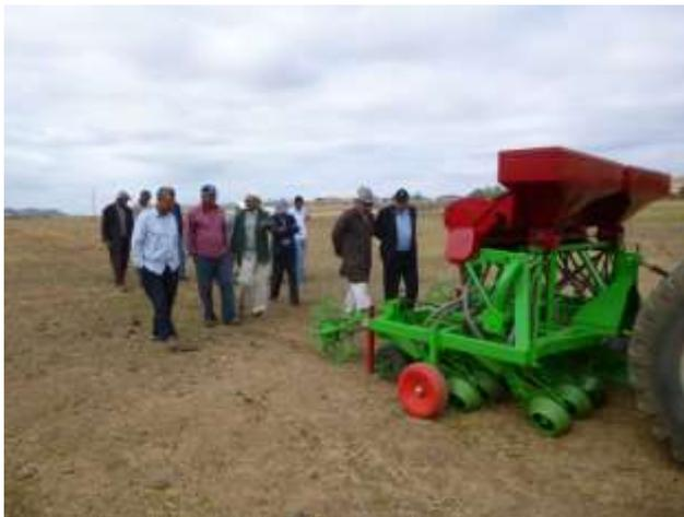
Angled single disc as fitted to seed drill on 4WT
