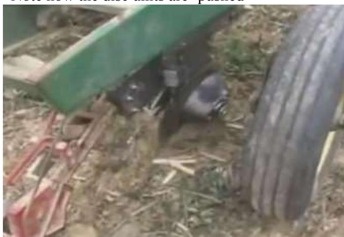
An angled single disc unit fitted vertically under a John Deere row unit
