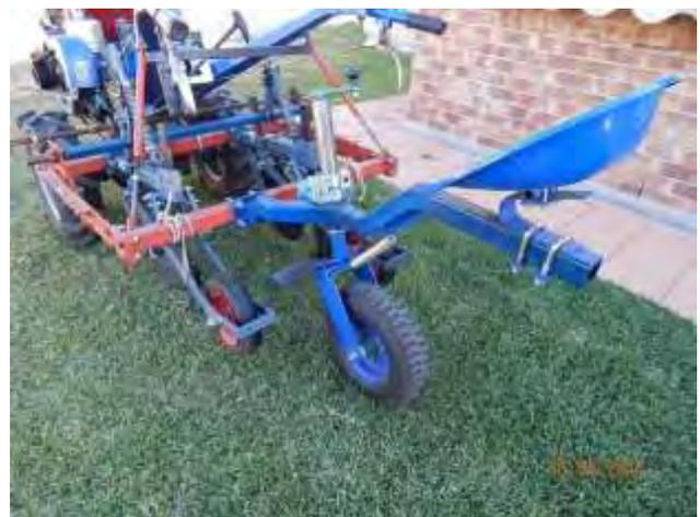
The left hand picture shows the raise-lower system with the pressure/helper spring. The control lever is yet to be constructed. Also a new seed box frame will be built so that it does not hinder any of the mechanisms. Note that the tine assemblies are adjustable for row (line) spacing which is variable from 60-90 cm row width.
