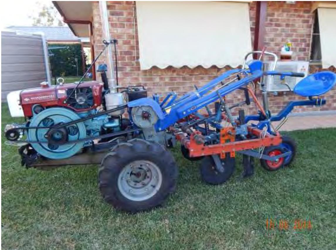
This shows the complete setup with the tines attached to the tool bar. Each assembly must be compact, to fit between the front and rear tool bars, and yet not be obstructed by the handlebars or other parts of the 2WT.
