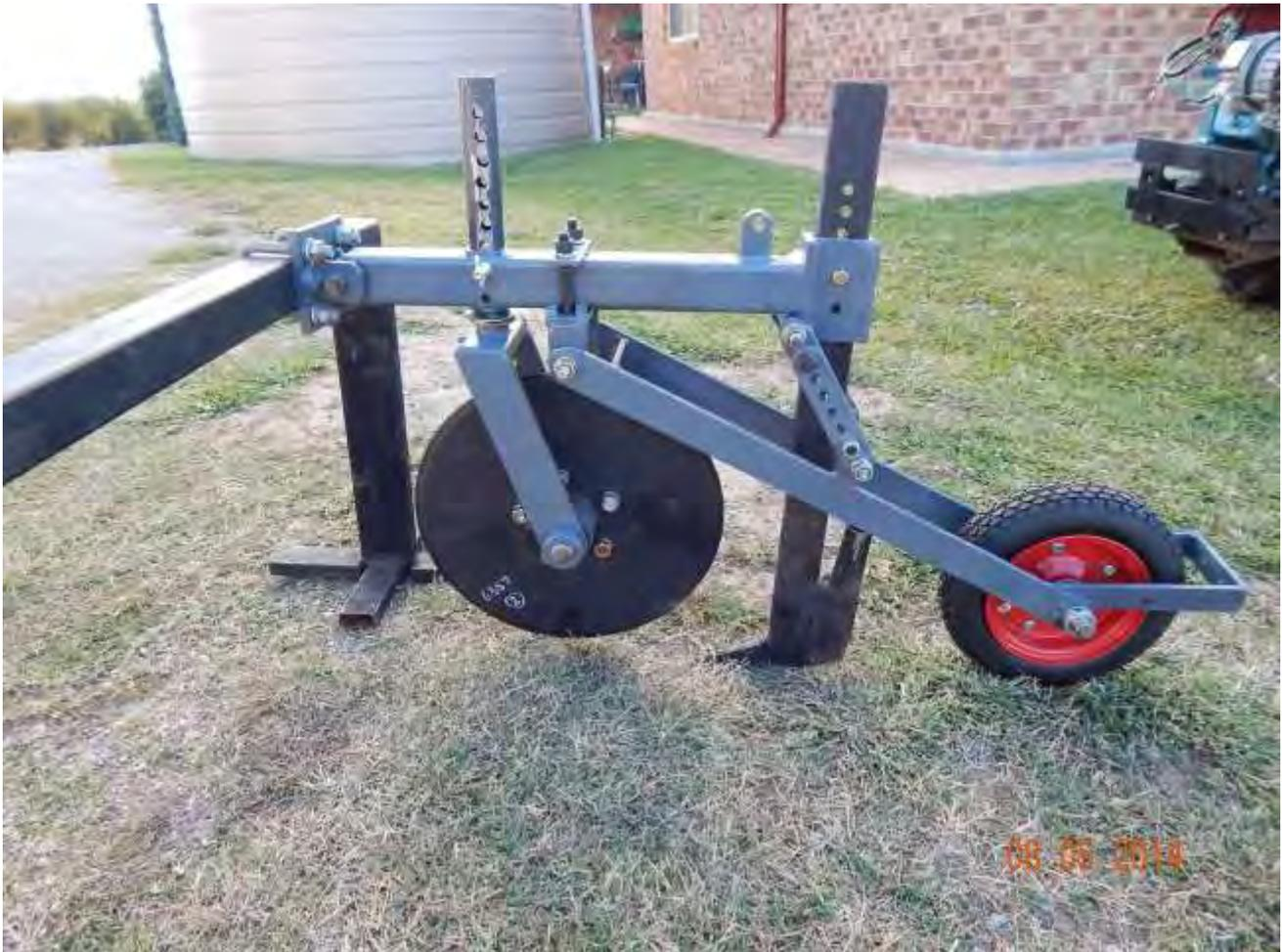
This shows a complete tine unit, complete with the optional cutting coulter. The tine is a standard 50 x 12 hi tensile steel piece, with non-detachable hard faced point. Point rake angle is 30 degrees to minimise draft. The cutting coulter is 356mm (14 inches) in diameter, and swivels. The camber angle of the yoke for the coulter is 20 degrees (with a larger camber angle the coulter has insufficient clearance to the tine).
