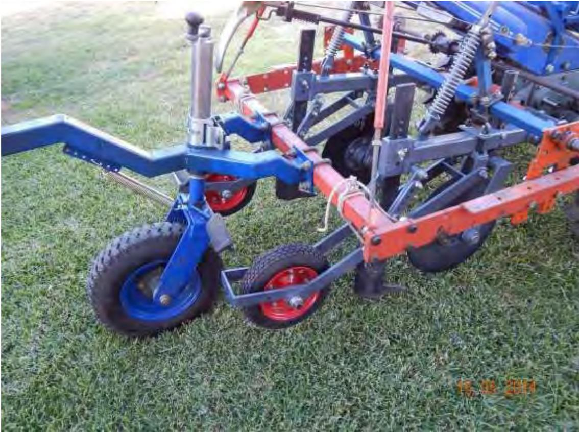
This is a right hand rear view of the complete assembly. The lift system is yet to be completed, along with the seed box frame and seed and fertiliser metering units.
