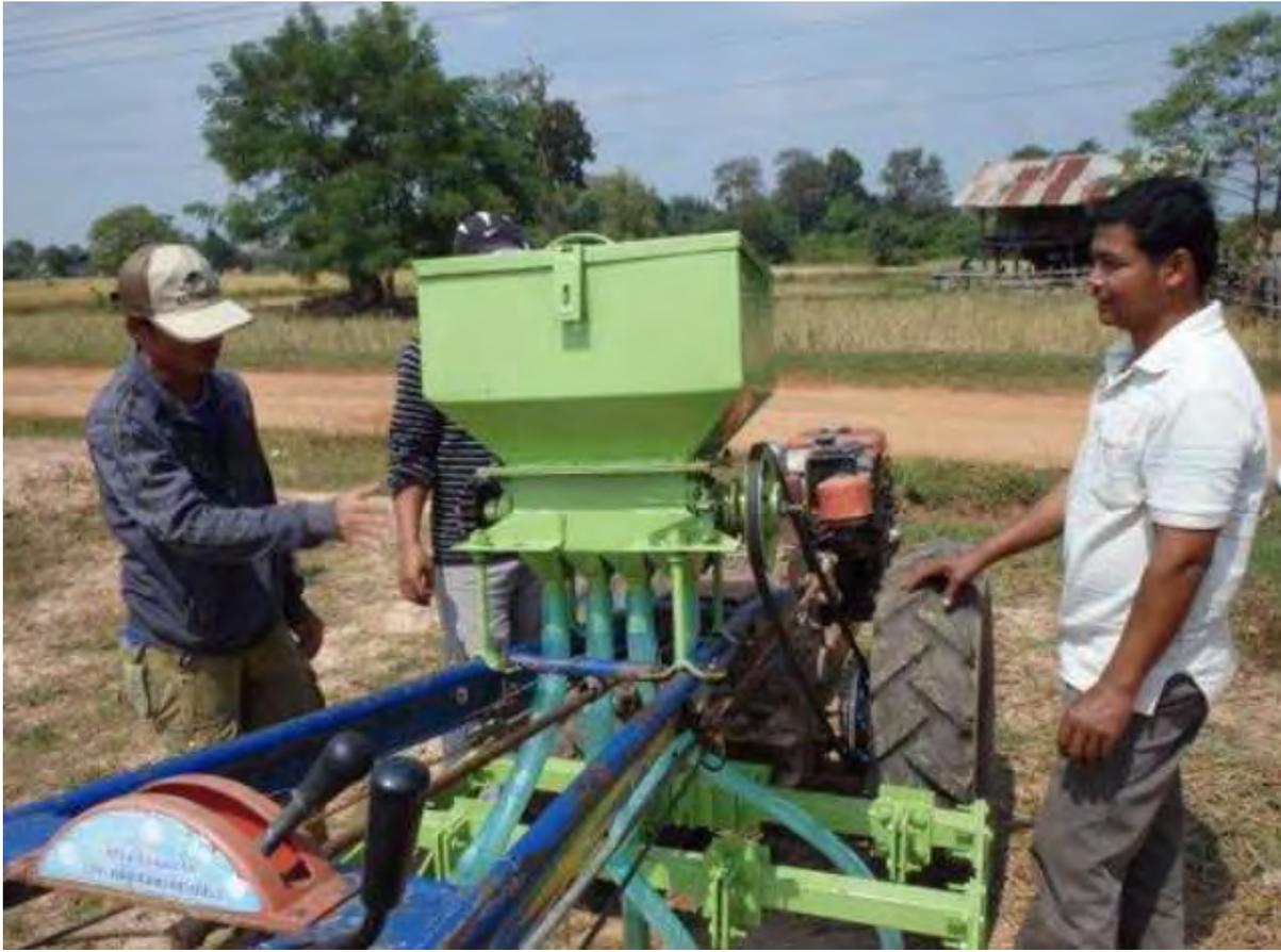
Related to the above unit, Dr Leigh Vial of IRRI has developed a modified form of the Thai direct rice seeder that allows placement of fertiliser in line with the direct seeded rice. This seeder has design features from the original ACIAR-Rogro two wheel tractor seed drill (now the ARC Gongli), as well as the Thai built unit.
