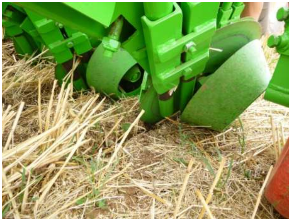
A close-up of the angled disc, showing the seed and fertiliser tubes and the depth/gauge wheel
