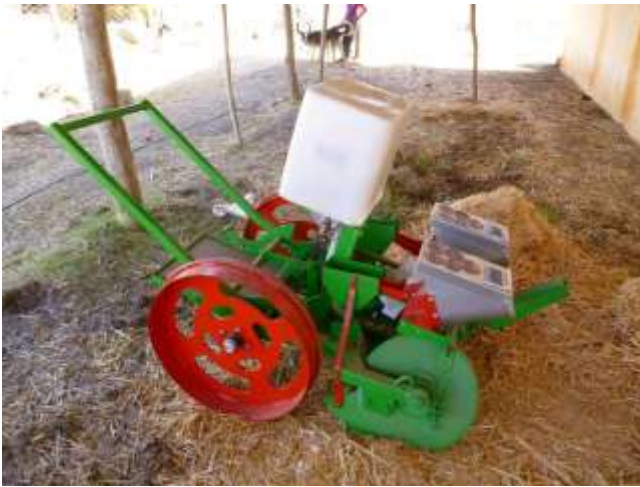
Angled single disc seed drill (two row) for animal traction (and perhaps 2WT)
