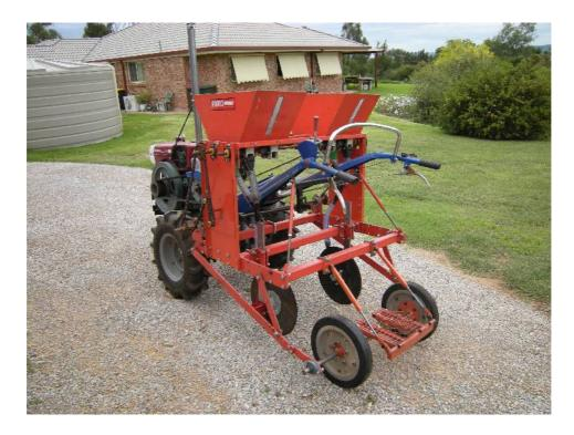
This is my first attempt at fabrication of a single disc undercarriage to fit to a 2WT. The discs are 40 cm (16") in diameter and 4mm thick. Each disc is set at 5 degrees of offset, and no tilt (undercut). Each disc assembly fits into the tine frame and clamp, with a similar depth control mechanism to that for the standard tine. It has yet to be tried in the field.
