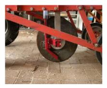
Apparently some Australian farmers are making their own 'Discamate' style units .I made up this single disc opener using this idea at an estimated cost of \$150. I have used a stub axle and hub from a box trailer (\$90) and fitted a double bevelled coulter disc (\$45). The delivery tube was made up in the workshop. This is what is fitted to the seed drill shown above. Note the operator platform also fitted, as well as the larger press wheels. Perhaps this style of unit is affordable.
