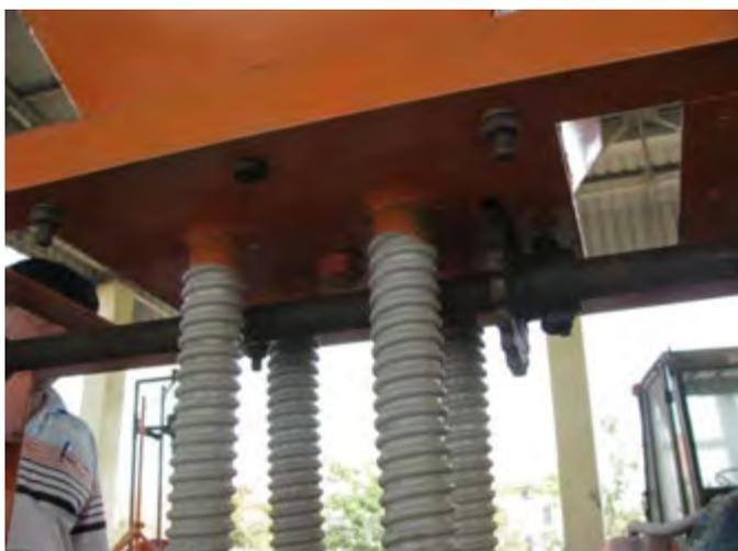
A view from the underside showing the drive mechanism for the horizontal plate. Apparently each plate meters seed to four outlets.
