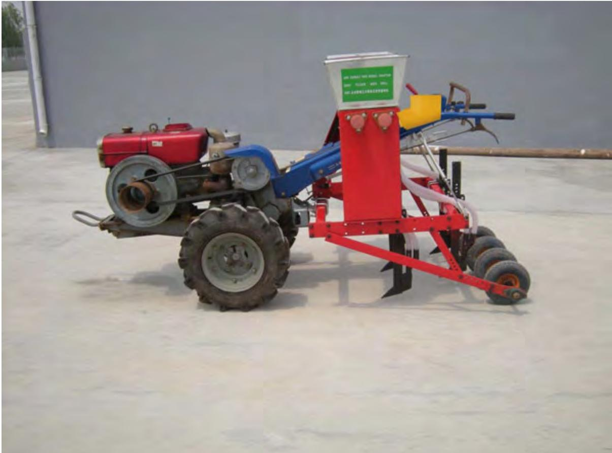
An ARC Gongli 2WT seed drill with the optional inclined plate seed meter fitted.
