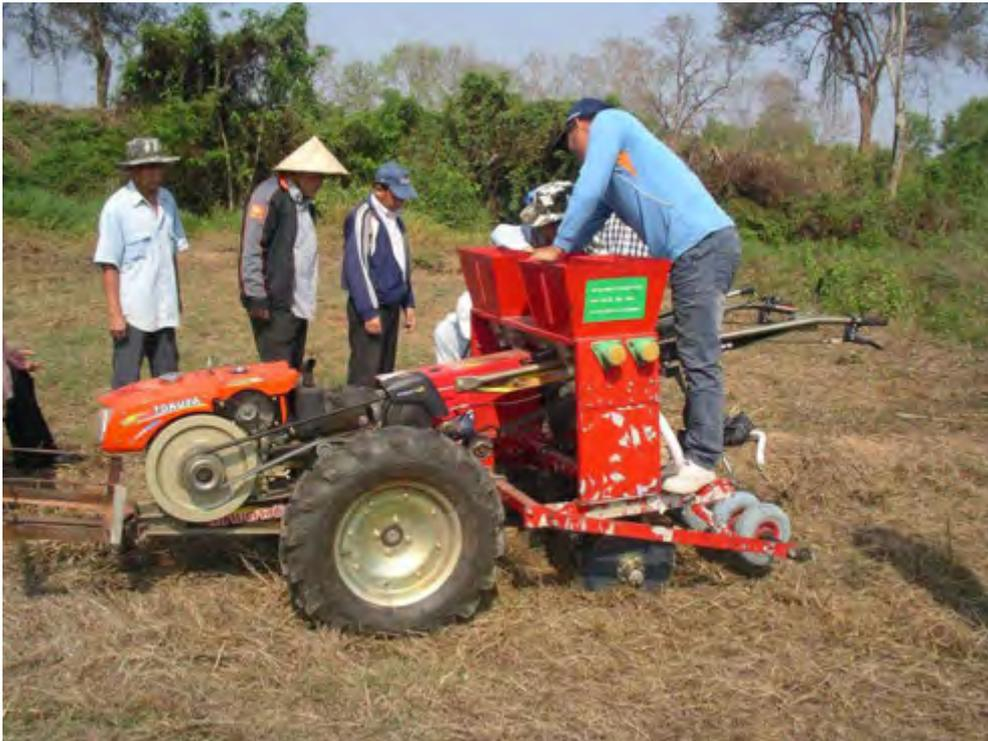
The ARC Gongli fitted to a Thai made 2WT (note the weight box on the front)
