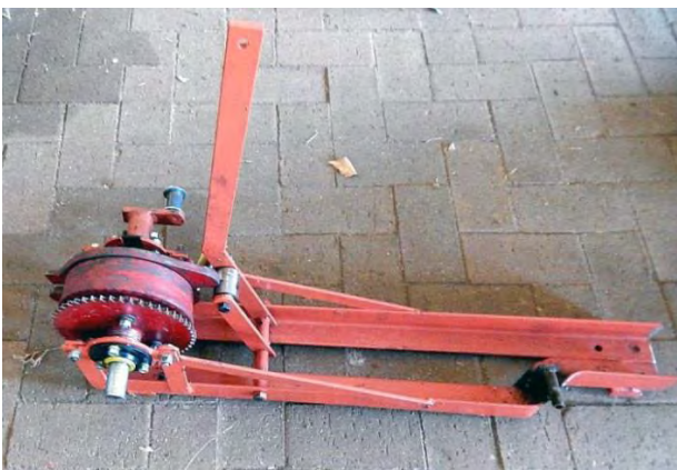
A mechanical ‘rope trip lift’ from a 1930’s Seed drill
