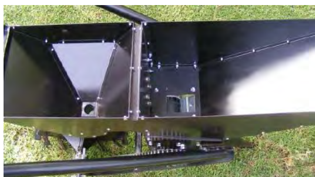
The seed and fertiliser boxes (left) and the tine assembly with steel drive wheel (right)
