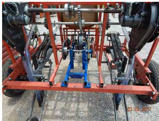
A modern version of the same lift fitted to a trailing 2WT two row planter
