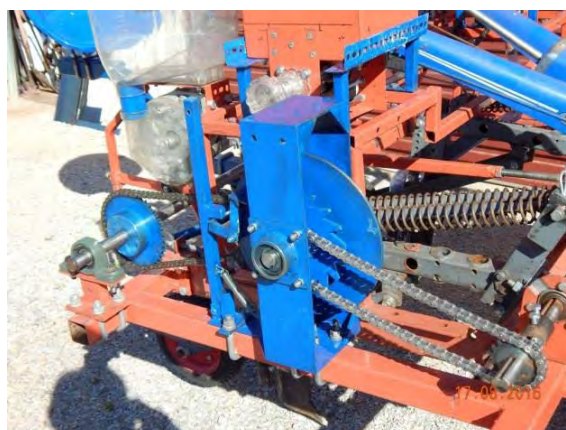
Another experimental lift operating on a single revolution ratchet clutch principle.
