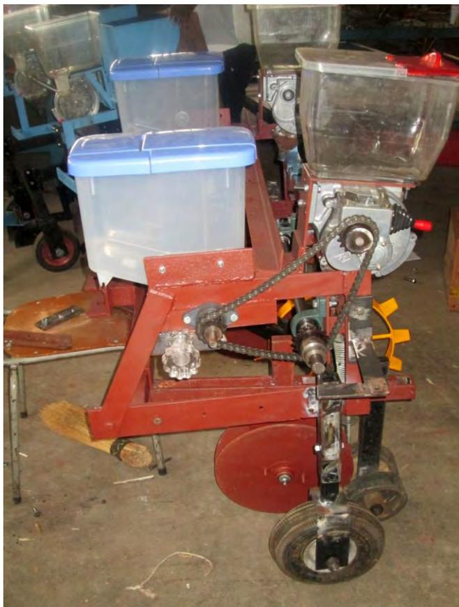
This planter is fitted with two Chinese made double disc soil engaging tools. These are on drag arms which are spring loaded.
