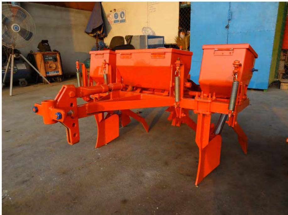
Clive Murray (Syngenta Foundation SE Asia) has supplied me with two pictures of a Thai made 2WT planter. I do not have any detailed information on this planter. However it appears to be fitted with a pair of inclined plate seed metering systems on the seed boxes. The seed covering devices and the drive system is clearly visible.
