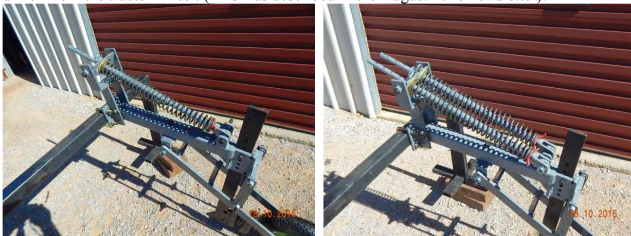
Spring loaded tine with single spring (left) and double spring (right)
