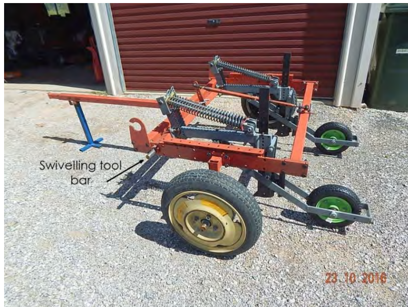
Side view of the frame, showing two tine assemblies, and swivelling tool bar.
