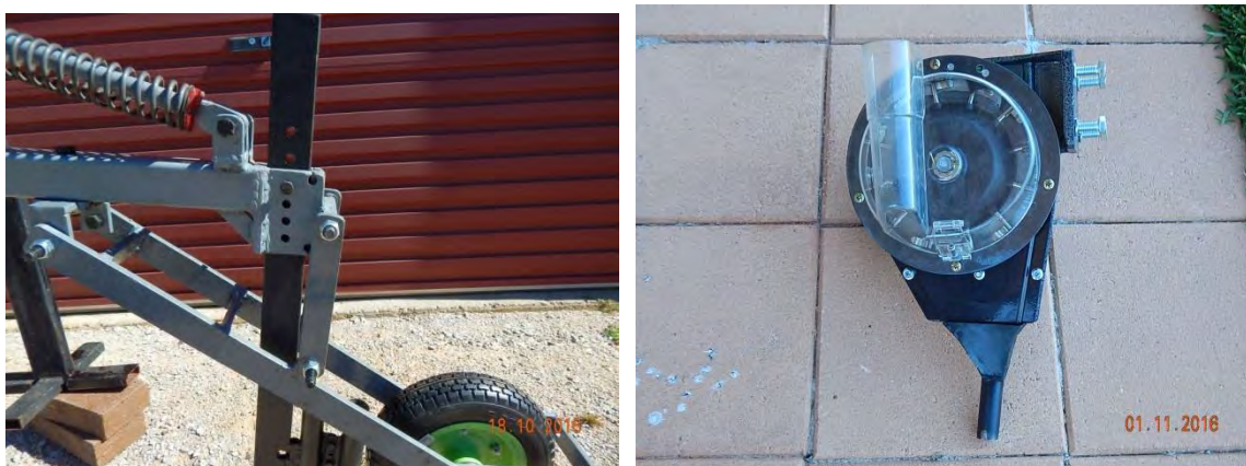
A tine shank showing depth adjustment (left) and a finger pickup seed meter (right) (The seed meter has a non-standard seed delivery tube.)
