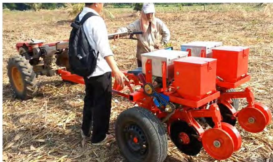
No specific details are available at this time for these planters. However I note that they are disc units, and in my opinion will need extra weight for proper penetration in all but very soft soils. My guess is that they are fitted with inclined plate seed meters. I can forward a copy of the brochure to anyone who is interested. The Thai manufacturer also makes larger planters of similar design for 4WT.
