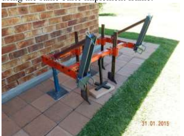
The alternative tool bar for cereals (left) and the rope trip lift mechanism (right)
