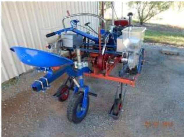
Rear view showing the widened tool bar with seed boxes beside the handlebars (left) and the swivelling tool bar to raise and lower the tines or discs (right)
