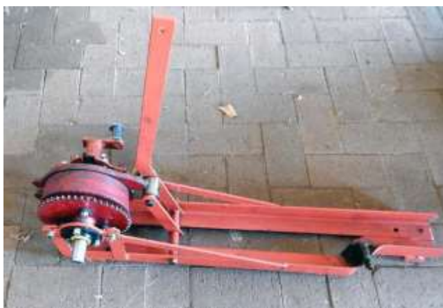
The alternative tool bar for cereals (left) and the rope trip lift mechanism (right)
