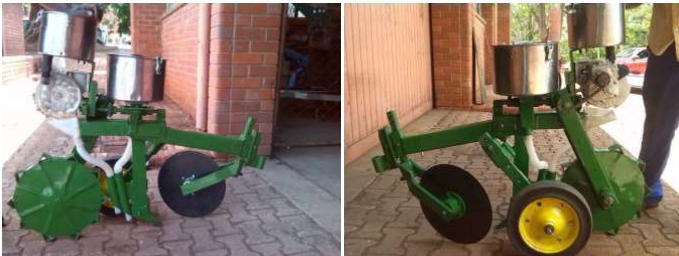
The Fitarelli/Grownet single row 2WT seed drill
