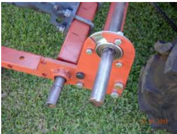
Rear view showing the widened tool bar with seed boxes beside the handlebars (left) and the swivelling tool bar to raise and lower the tines or discs (right)
