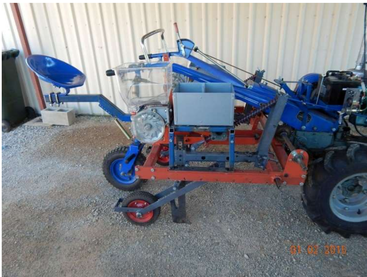
The latest prototype of the Gongli Africa Mark 2 showing the three seed boxes and the contour following tines.
